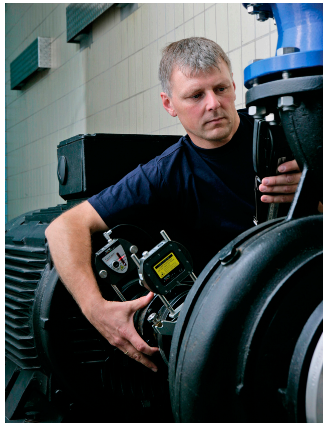
Alignment labor for an end-suction frame-mounted pumps can be time-consuming and costly.
