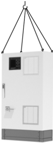
Fig. 1 Correct lifting of control cabinet
