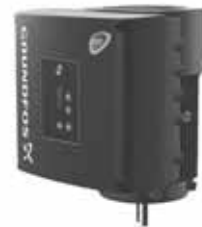
Fig. 3 Range of MLE motors 3x460-480 V, 20-30 Hp are induction style motors and have IE4 efficiency rating. MLE motor with a total efficiency exceeding the EuP IE5 up to 15 Hp (11 kW) and IE4 from 20 Hp (15 kW) to 30 Hp (22 kW) levels according to IEC 60034-30-1.
