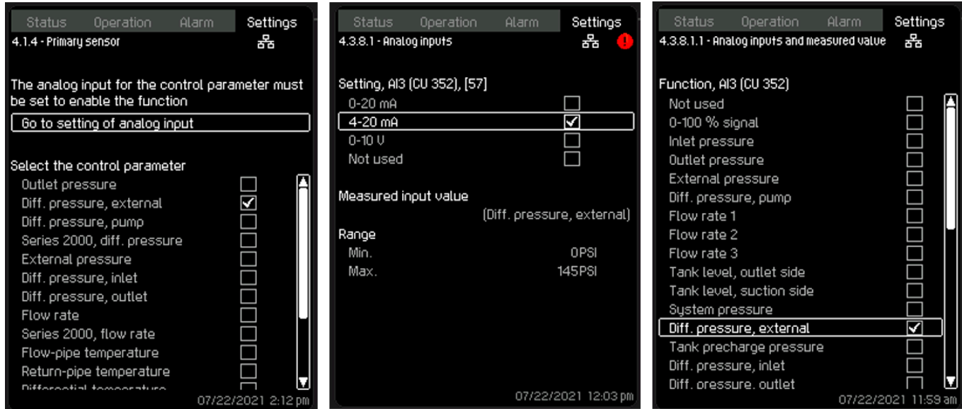
Figure 9: Setting up remote dP as primary sensor
