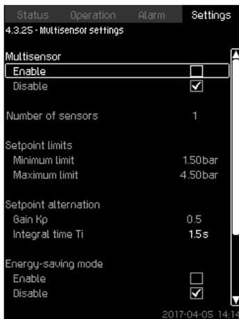
Fig. 104 Multisensor settings
