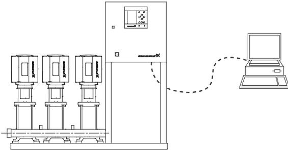
**Fig. 30** Pump system with external controller (open loop)
