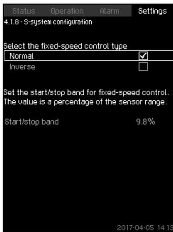
Fig. 57 S-system configuration
