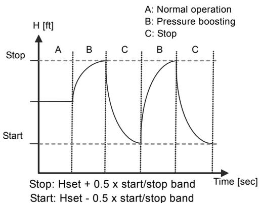
Fig. 74 On/off operation
