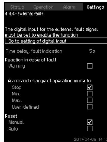
Fig. 113 External fault
