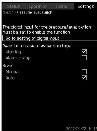
Fig. 108 Pressure/level switch
