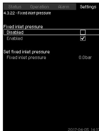
Fig. 101 Fixed inlet pressure
