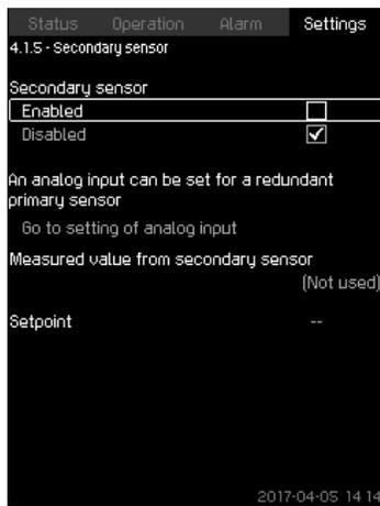
Fig. 52 Secondary sensor
