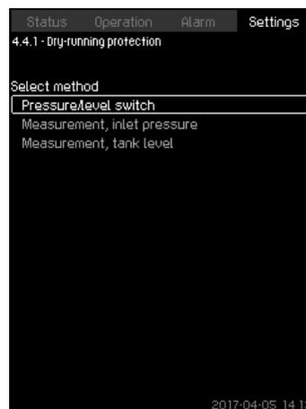
Fig. 107 Dry-running protection
