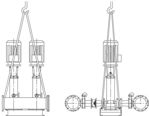
Fig. 5 Correct lifting of Hydro MPC XL
