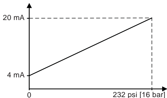
Fig. 35 Pressure response of RPI 0-232 psi
