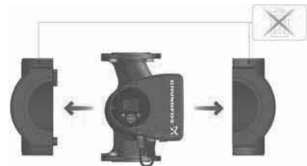
Fig. 3 Fitting insulating shells to the pump
